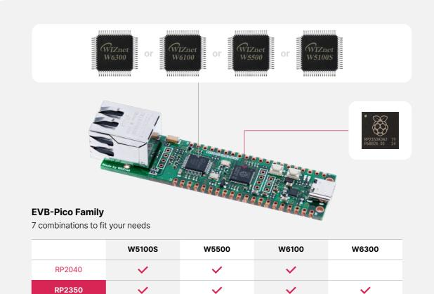
The **WIZnet EVB Pico 2 series** is designed to simplify and enhance Ethernet connectivity in embedded systems. By integrating WIZnet's industry-leading Ethernet controllers (W6100, W5500, and W5100S) directly onto the board, these evaluation boards eliminate the need for additional components or connections, offering a streamlined solution for developers.
