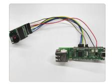
Integrates Arducam's 2MP module with a custom webserver on the W55RP20-EVB-Pico, enabling high-resolution image capture and chunk-based data delivery. Designed with robust buffer management, it smoothly handles large JPEG files—laying the groundwork for advanced camera features, dual-core operations, and potential live streaming extensions in future updates.
